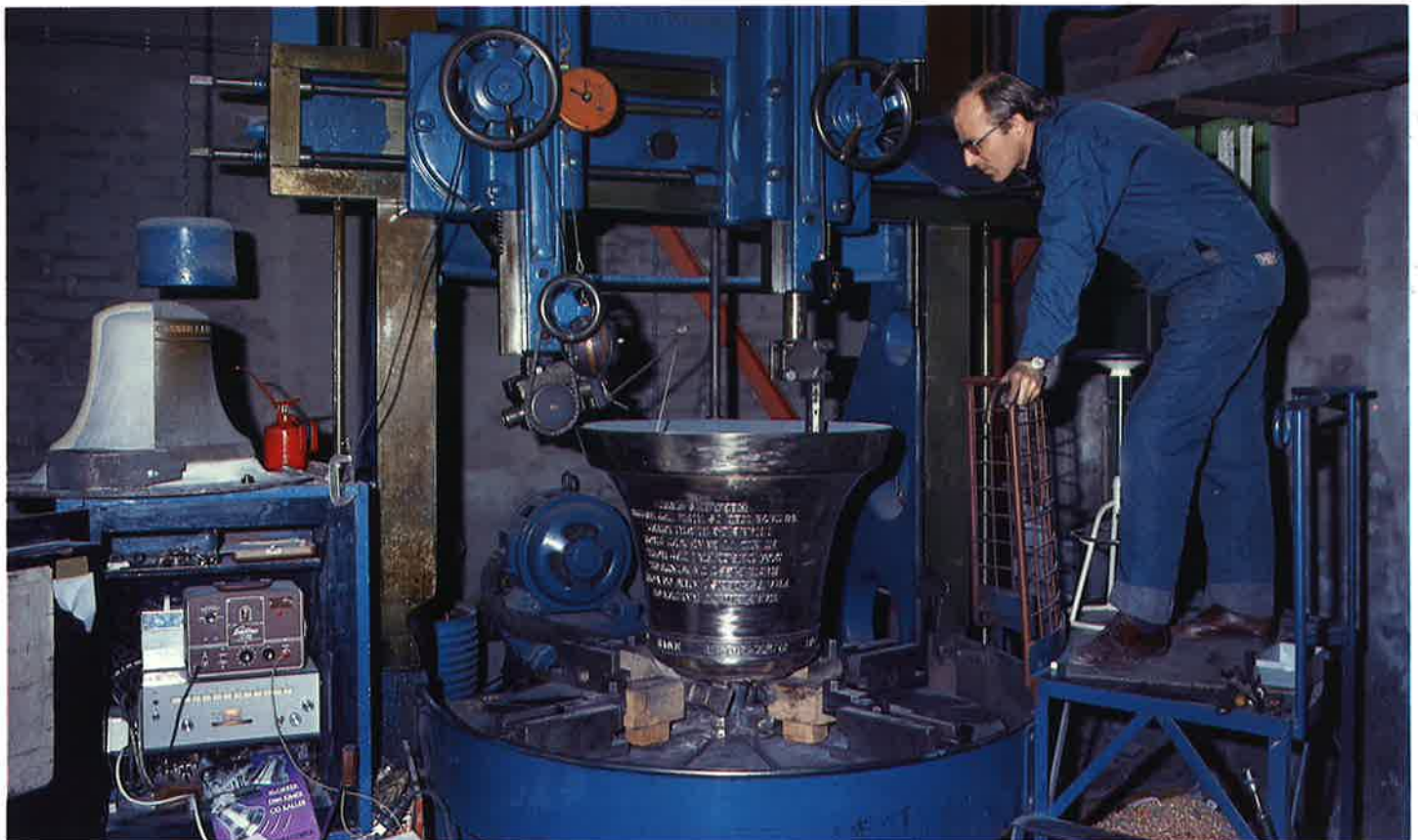
Klokken stemmes ved innvendig avdreining. The bell is tuned by removing metal from the inner surface by turning.
