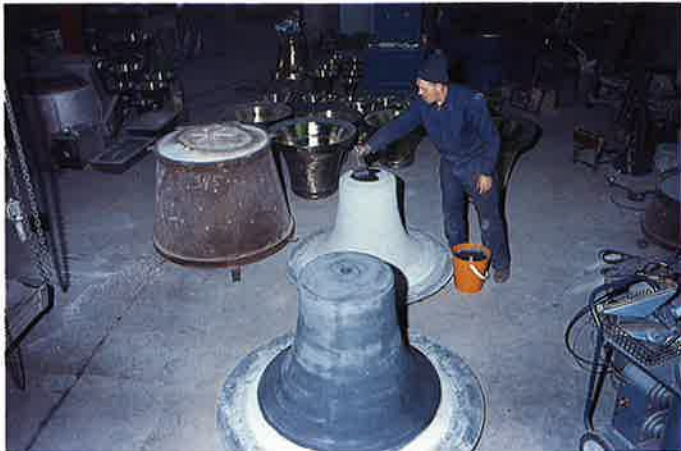
Form ferdig til å settes sammen. The mould is ready for assembly.
